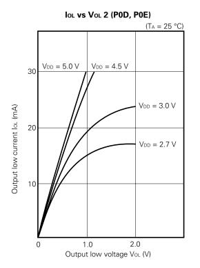
Caution The absolute maximum rating of the current is 30 mA per pin. The input voltage or output voltage of the P0E 1 pin must not be higher than 1⁄20 + 0.3 V.
